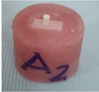
Figure 1: Resin cement cylinder bonded to zirconia plate after cutting the tube.
