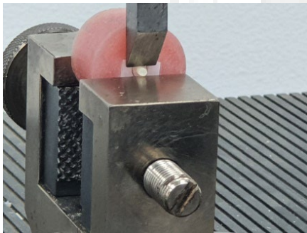
Figure 2: Shear bond strength test.
