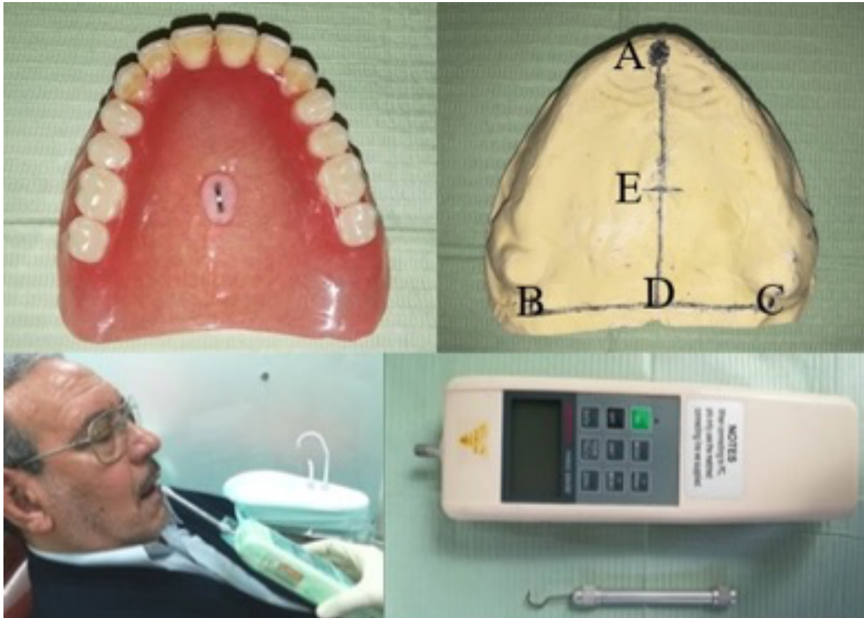
Fig. (6): Location of the geometrical center of the arch, stainless steel hook attached to the upper denture, Digital force gauge HF-100
