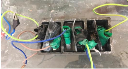
Fig. 3 Battery with electrodes made of composite foams
