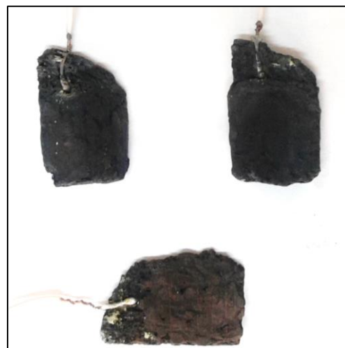
Fig. 2 Formed positive (one lower) and negative (two upper) electrodes made of composite foams
