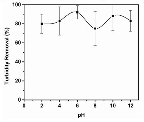
Fig. 3. Influence of water pH on turbidity removal.
