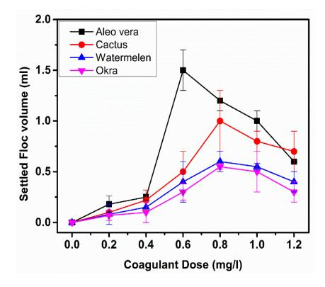
Fig. 1. Settled floc volume at various doses of different natural coagulants.
