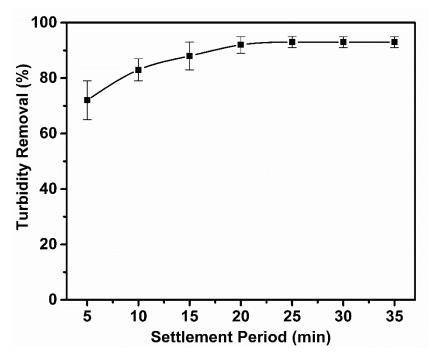
Fig. 7. Effect of settlement period on turbidity removal
