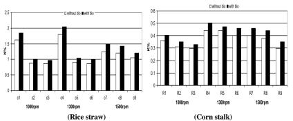
Fig. 4. Effect of chopping machine rotation feeding rates and biofertilizers application on K%, of the matured compost for rice straw and corn stalk
