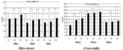
Fig. 2. Effect of chopping machine rotation, feeding rates and biofertilizers application on C/N ratio, of the matured compost for rice straw and corn stalk
