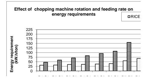
Fig. 1. Effect of chopping machine rotation and feeding rate on energy requirements of rice straw and corn stalks
