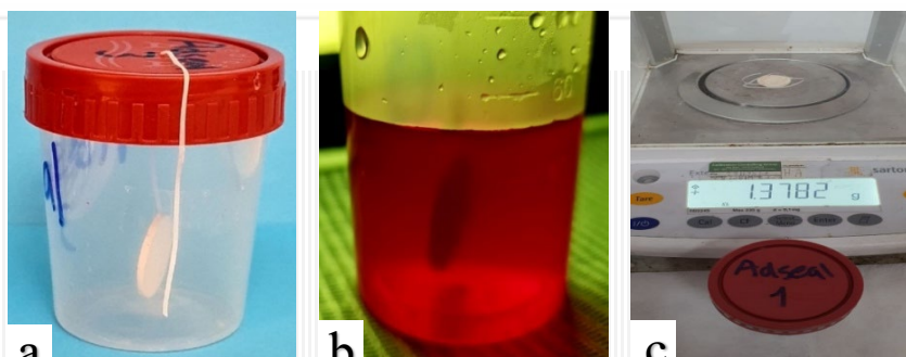
Figure 2: a. Hanging of the discs from the floss without touching the walls of the container. b. The plastic container filled with 50 ml HBSS and the sample hung in it. c. Weighing of the sample placing it and the floss in the center of the precision balance.
