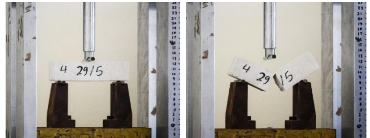
(a) (b) Figure (13): Compressive strength test of mortar samples according to ASTM ;(a) Testing samples, and (b) Mode of failure
