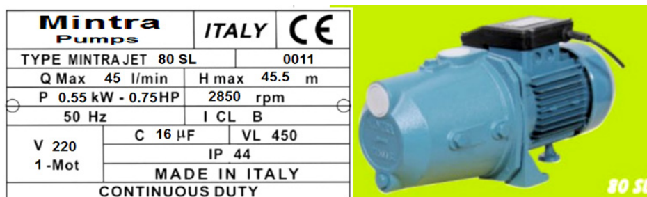
Fig. 1. Specification of the used water pump [1 inch 0.75 hp suction pump]. Knowing that 52.16 L/min is the actual measured pump's flow rate when the height equals zero.
