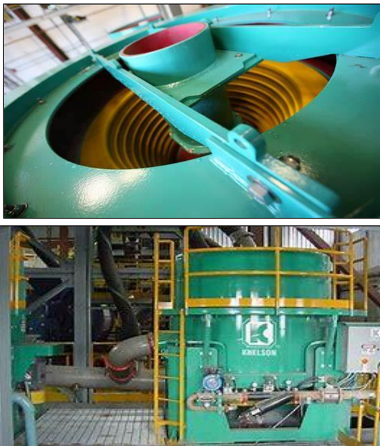
Fig. 11 Industrial Knelson Concentrator installed at Asanko Gold in Ghana.
