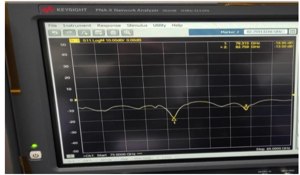
Fig. 22. S11 value at the screen of VNA
