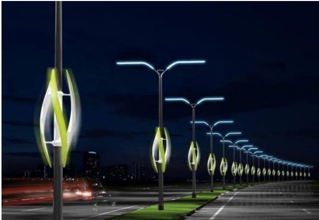
Fig. (9) Turbine Light Highway Lighting columns highways; in the idea depends on the exploitation of wind energy in operation instead of the electric energy consumption. The idea is to exploit the moving air resulting from vehicular traffic in highways and is absorbed to generate energy through which it operates and to illuminate
