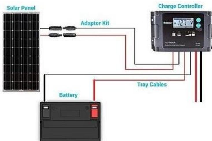
Fig. 4. PV system diagram.
