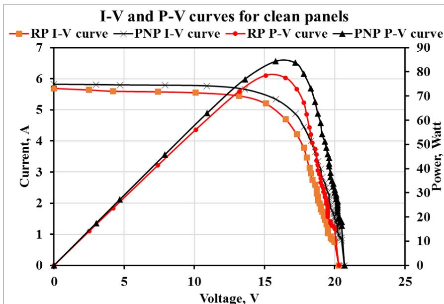
Fig. 7. The I-V and P-V curves for clean RP and PNP.
