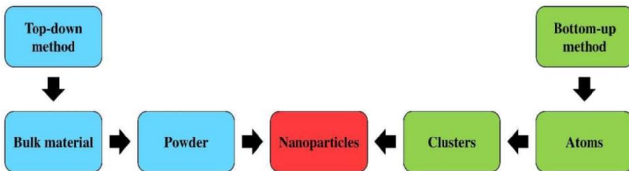
Fig. 2: The nanoparticles synthesis process.
