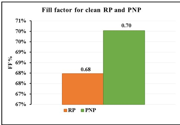
Fig. 8: Fill factor for clean RP and PNP.
