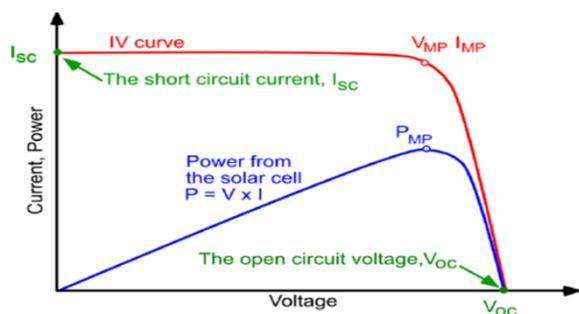
Fig. 1. I-V and P-V curves for solar panel (Alzahrani et al., 2020).
