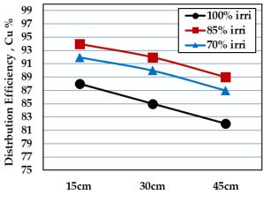
Drip line depth (cm) for Leaky-pipe
