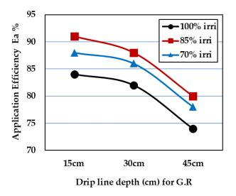
**Fig. 4.** Application Efficiency (Ea %) for all irrigation levels and different depths for G.R.
