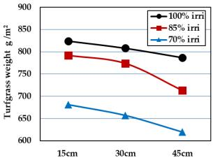
Drip line depth (cm) for Leaky-pipe
