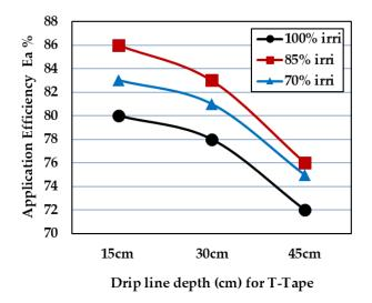
**Fig. 3.** Application Efficiency (Ea %) for all irrigation levels and different depths for T-Tape.
