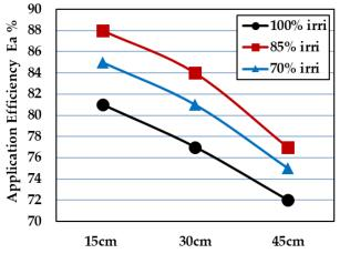
Drip line depth (cm) for Leaky-pipe
