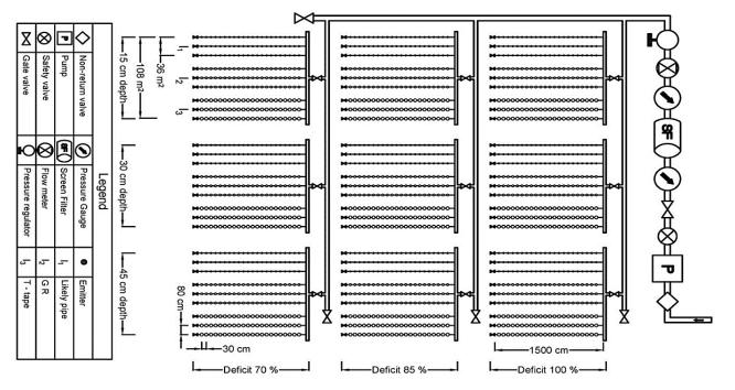
Fig.1. The layout of the experimental field irrigation treatments and replicates.
