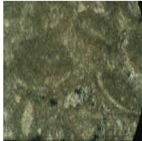
Fig . 47. display thin section of limestone from another local quarries in the calcareous lower Eocene plateau (cross Nikol)( C.N) (x 4) which exhibits the same
