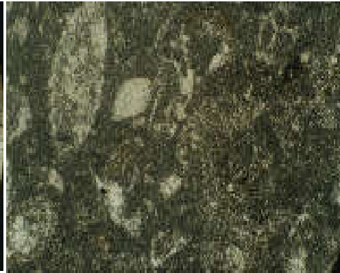
Fig.45 display thin section of limestone from archaeological buildings in Abydos (cross Nikol) ( C.N) (x 4) (microscope which exhibits Nummulitic limestone (Thebes formation) which contains algae and a few fossils voids , and the main component Micrite , indicating to similarity in structure , , composition and features to the limestone from local quarries in the calcareous lower Eocene plateau
