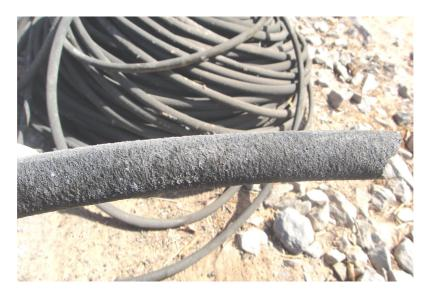
Fig. 2. The subsurface drip leakage lines
