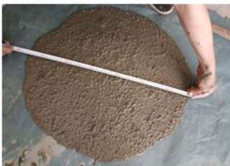
Fig 2. Concrete measurement diameter
