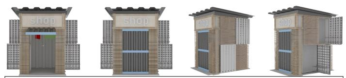
Figure 11: A model of the proposed commercial unit and the method of opening and closing it.
