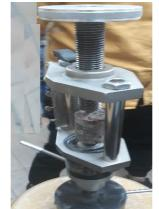
Fig. 6 Photograph showing the Point load test system
