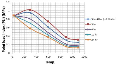
Fig. 7. Variation of the (PLI) (MPa) of Sandstone rock for different temperature degrees in different cases
