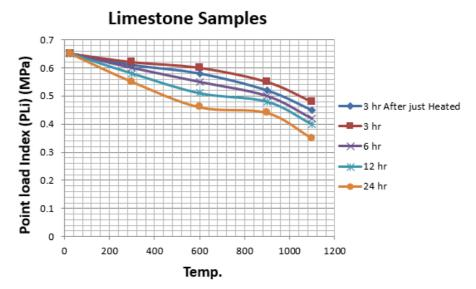
Fig. 8. Variation of the (PLI) (MPa) of Limestone rock for different temperature degrees in different cases
