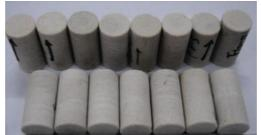
Fig. 5 Shape of the Cylinders Samples of Marble rocks
