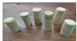
Fig. 4 Shape of the Cylinders Samples of Limestone rocks
