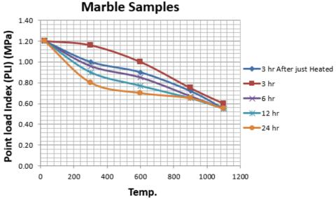
Fig. 9. Variation of the (PLI) (MPa) of Marble rock for different temperature degrees in different cases
