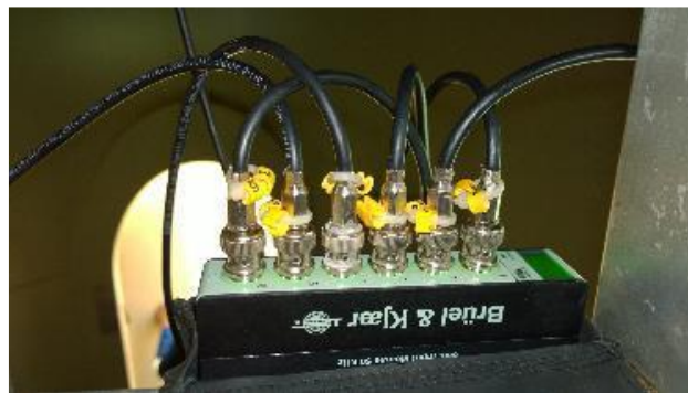
Fig. 4: Test equipment (a) LAN-XI unit attached to the ladder
