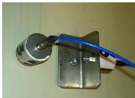
Fig. 4: Test equipment (b) PCB accelerometers with magnetic mounting attached to the tower wall
