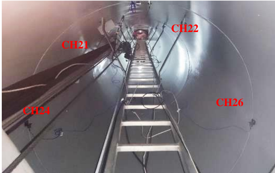
Fig. 6: Accelerometers arrangement at level 2 for Vestas N47 Test Setup
