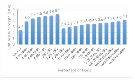
Fig.8 Indirect tensile strength values of the investigated mixes.
