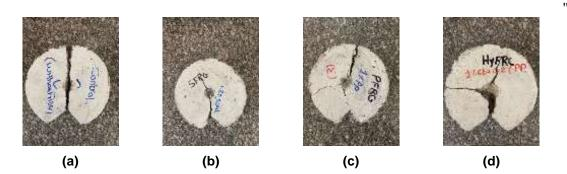
Fig.11. Failure pattern of the geopolymer concrete specimen (a) Control specimen (b) SFRG (c) PFRG (d) HyFRG
