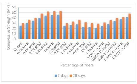
Fig. 7: Compressive strength values of the investigated mixes.
