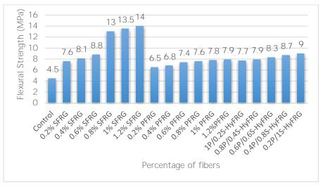
Fig.9: Flexural strength values of the investigated mixes.
