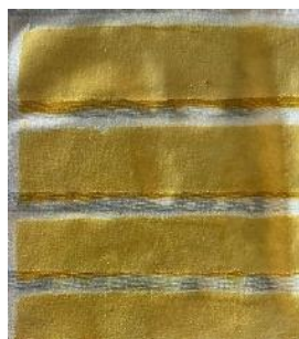
Pic.2 A wet polyester sample printed a hydrochromic paste
