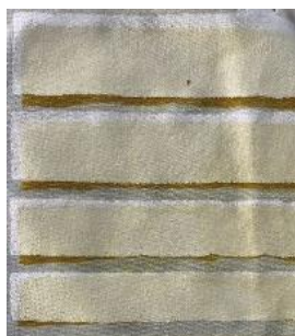
Pic.1 A dry polyester sample printed a hydrochromic paste
