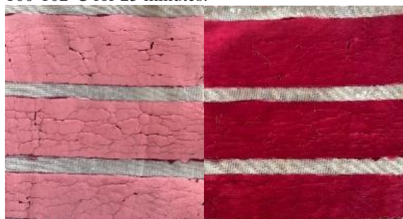
Pic.1 A dry polyamide sample printed a hydrochromic paste
