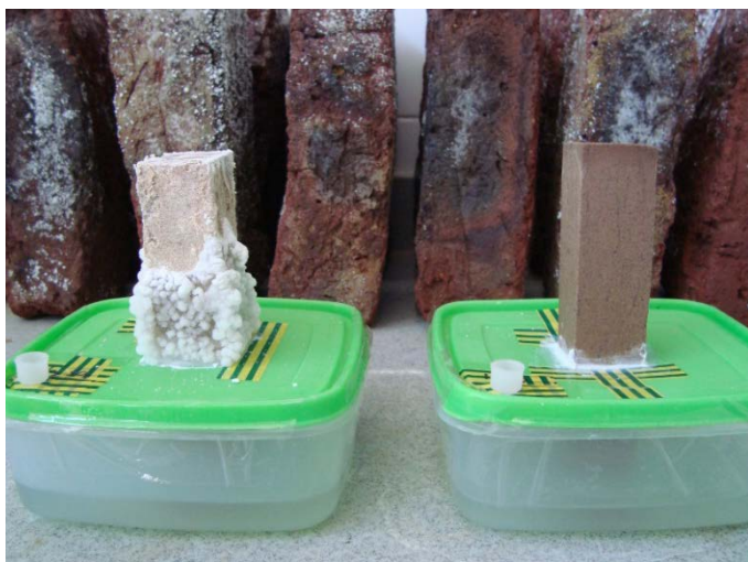
Fig. 1: Experiment on the effects of groundwater on sandstone sample (left) and potable water (right)
