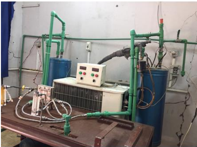
Fig 2: Real photo of the AGMD experimental setup
