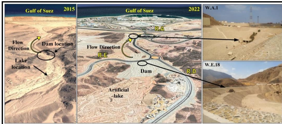
Fig. 29: Methods of Protection against the Hazards of Flash Floods of W.E.18 and W.A.1 Basins
