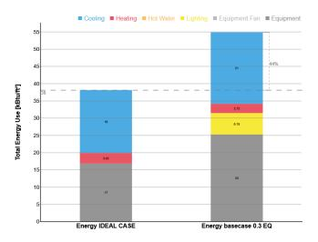
Figure 15: (Total energy use intensity kwh/m<sup>2</sup> ) Comparison chart for IDEAL case and base case
