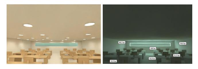
Figure 14: Rendered shot of the lab. After applying TDDs
