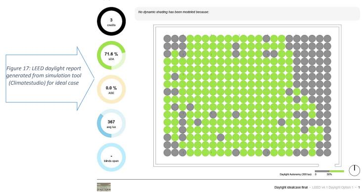
Software: ClimateStudio v1.9.8306.17105 Engine: Radiance 5.3 Weather: EGY\_QH\_Cairo.West.AP.623680\_TMYx.epw North Offset: 0° Ambient Bounces: 6 Passes Completed: 100 Primary Ambient Samples: 6400
