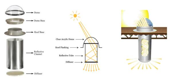
Figure 8: Tubular daylighting device component
