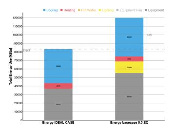
Figure 16: (Total energy use kw/h ) Comparison chart for IDEAL case and base case
