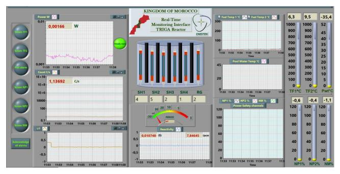
Fig. (3): Live Data Screen with all necessary data to perform the experiments
