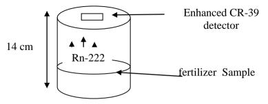
Figure (3): A schematic diagram of the sealed –cup technique in fertilizer sample.
