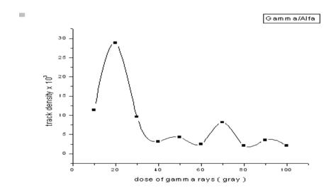
**Figure (1)** Variation of track density with the pre gamma dose 24 Vol.35, No.1, Spt., 2016
