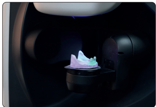
Fig. (2): Scanning of Cobalt chromium bar-abutment assembly
