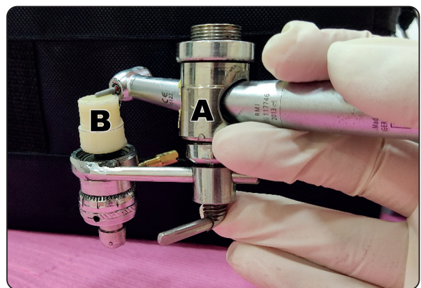
Fig. (1): (a) The first part for holding the high-speed handpiece to be fixed during the grinding, (b) the second part was a teflon mold for holding the sample and can be rotated around its long axis.
