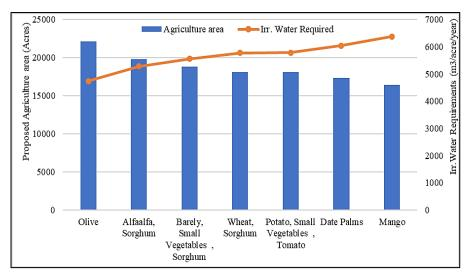
Fig. 6: Proposed cultivation area and irrigation water requirements
