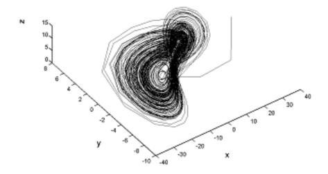
Figure 3: Hyperchaotic attractor of the novel fractional order hyperchaotic system with commensurate order  $\alpha = 0.97$  and  $\sigma = 35$ ,  $\eta = 4$ ,  $\rho = 25$ , d = 5,  $\mu = 35$  and  $\nu = 100$ .
