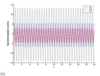
Figure 4: Shows the synchronization errors between the drive and response systems (5.1) and (5.2) using the controllers (5.4) and feedback control gains  $k_1 = 2$ ,  $k_2 = 4.3783$ ,  $k_3 = 1$ ;(a) The synchronization errors converge to zero when using fractional order  $\alpha = 0.9$ ; (b) The synchronization errors do not tend to zero when using  $\alpha = 1$ .
