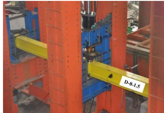
Figure 4: Test specimen and loading arrangement [21].
