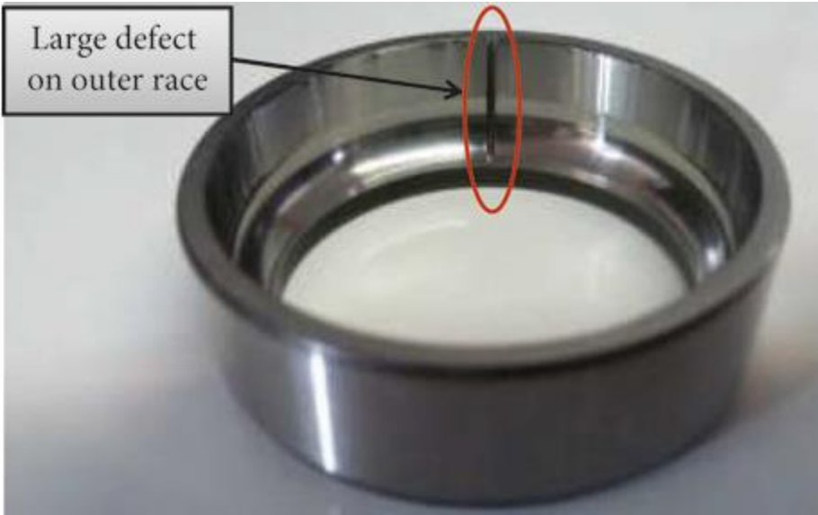
Fig. 2 Defects located in outer race of the bearing.
