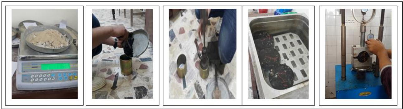
Figure (2): Preparing the specimen for Marshall Test
