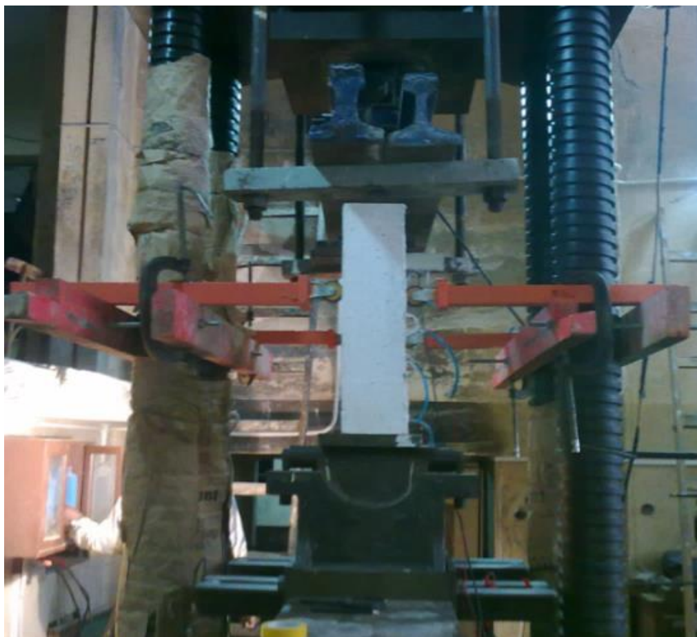
Fig. 2. Photo of the test setup and instrumentations (Side View) .
