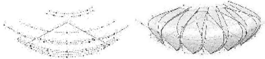
Figure 4: On the left the constrained points, on the right the control surfaces to generate the design variations of Hangzhou Tennis Center (Miller, 2011b)
