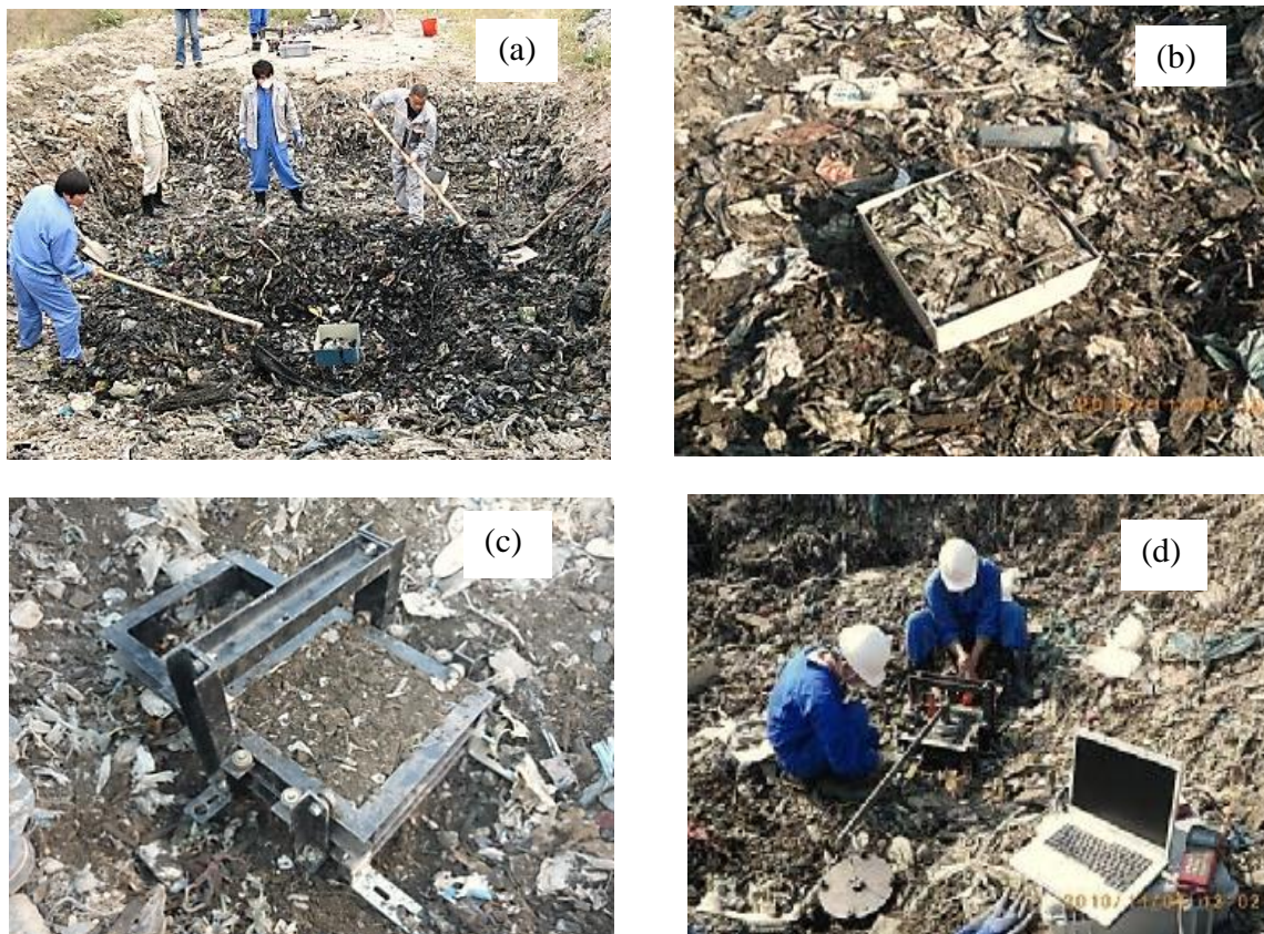
Figure 2. Steps of preparation of undisturbed specimen for in-situ direct shear test.
