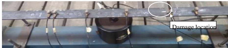
Fig.(19) Specimen D3;damaged at 0.68L
