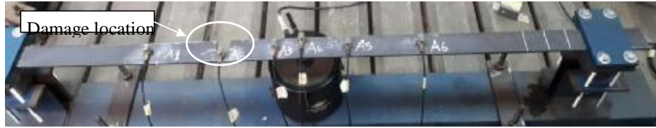
Fig.(18) Specimen D2;damaged at 0.37L
