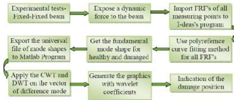
Fig.(1) General procedure adopted for the location of damage using wavelet analysis on the mode shape difference function
