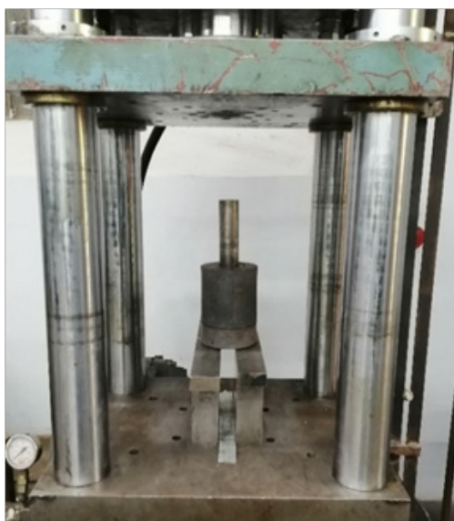
Fig. 2: The compacting rig and the hydraulic press
