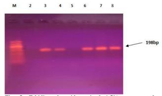
Fig. 5: Ethidium bromide stained 1.5% agarose gel electrophoresis showing: Lane 1: MW DNA marker of 50bp ladder, Lane 2: negative control. Lane3: positive control Lane 4, 6, 7, 8: positive isolates for icaD gene (198bp). Lane 5: negative isolate for icaD gene.
