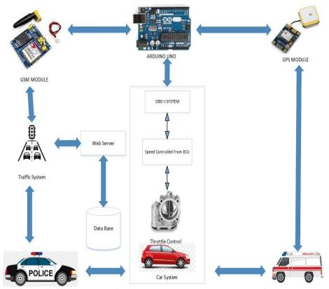
Fig (3) shown diagram of the proposed system and its components
