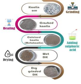
Fig.1: Production of alum and de-aluminated metakaolin [8]
