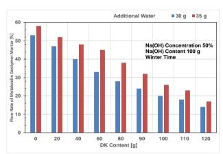
Fig. 5: Flow Rate of MK Geopolymer mortar for optimum contents
