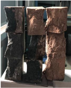
Fig. 22: Failure mode of compressive strength test
