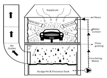
Figure 3: schematic for vehicle coating and VOCs pollutants release
