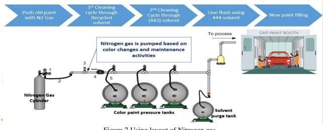
Figure 7 Using layout of Nitrogen gas
