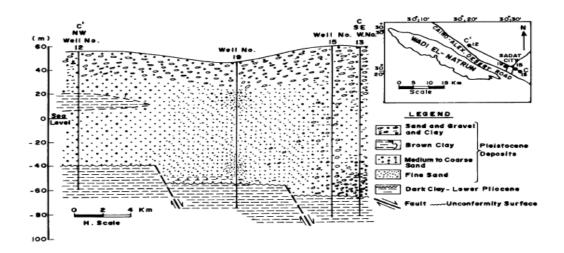
Fig. (2) Geological cross section  $C-C^-$  crossing the study area from the NW to the SE (El-Sayed 1999)
