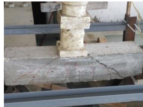
Figure 8: Failure of (CA)
