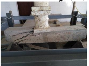
Figure 12: Failure of (CB)
