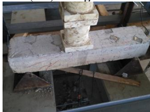
Figure 11: Failure of (CE)
