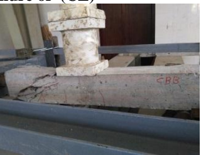
Figure 13: Failure of (CBB)
