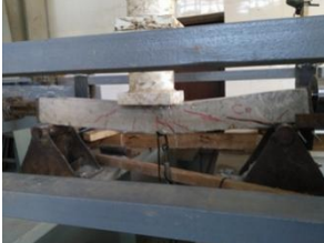
Figure 7: Failure of (C0)
