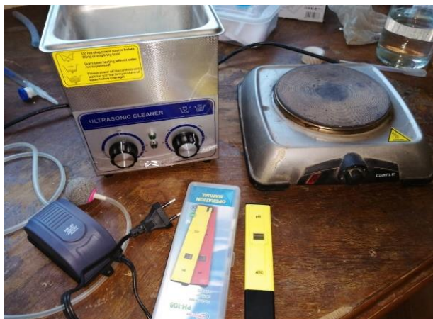
Figure (3) The apparatus required for ultrasonic process
