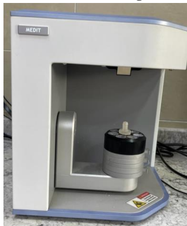
Figure (3): Scanning of the master die in Medit T-300 scanner
