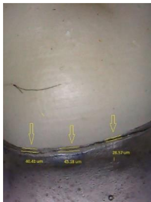
Figure (9) Representative microscopic image showing VM gap values for 120o group
