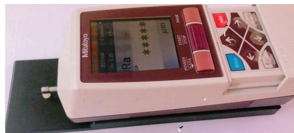
Figure: Surface roughness measured by a profilometer.
