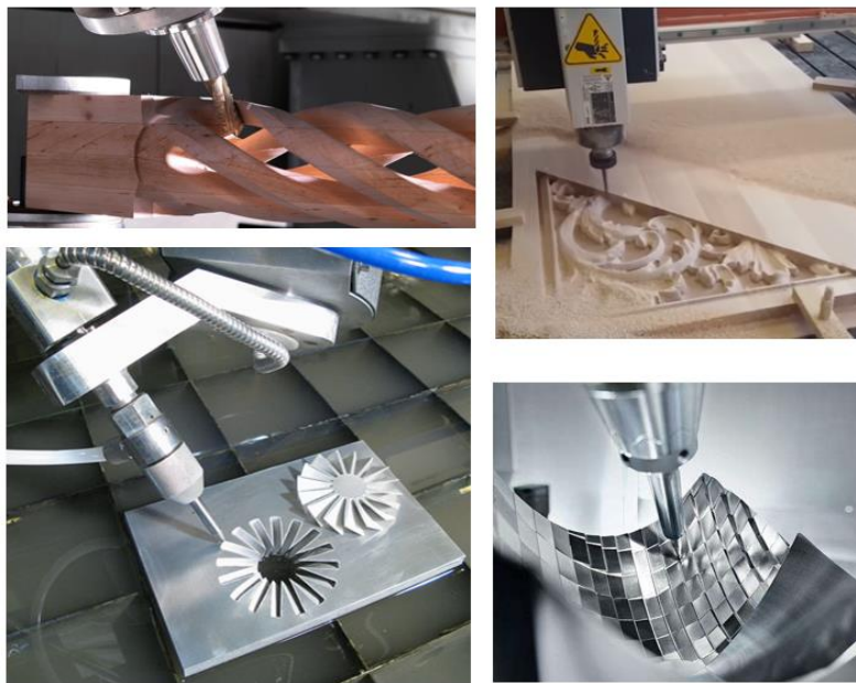
Fig. (10) Reveals the application of 5 axis CNR in wooden and steel parts
