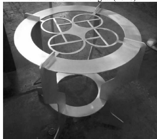
Fig. (7) Stainless steel Coffee table cut by plasma. (Fred P. Liza, Cameron B. Yao, Joein L. Luces, Vincent Boy E. Manabat, and Renann G. Baldovino. (2015))
